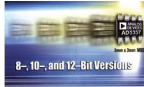
AD5337/AD5338/AD5339 are dual 8-, 10-, and 12-bit buffered voltage output DACs in an 8-lead MSOP package, which operate from a single 2.5V to 5.5V supply, consuming 250µA at 3V.
