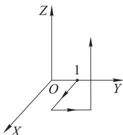
$$\begin{aligned} U(x, y, z) &= \int_0^x \left(2xz^3 + \frac{3z}{y^2}\right)_{y=1, z=0} dx - \int_1^y \left(\frac{6xz}{y^3}\right)_{z=0} dy + \\ &+ \int_0^z \left(3x^2z^2 + \frac{3x}{y^2}\right) dz = x^2z^3 + \frac{3xz}{y^2} + C. \end{aligned}$$
