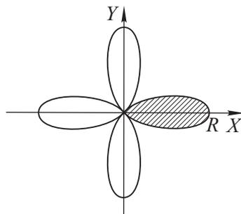
$$\begin{aligned} S &= \frac{1}{2} \int_{-\frac{\pi}{4}}^{\frac{\pi}{4}} R^2 \cos^2 2\varphi d\varphi = \frac{1}{2} R^2 \int_{-\frac{\pi}{4}}^{\frac{\pi}{4}} \frac{1 + \cos 4\varphi}{2} d\varphi = \\ &= \frac{1}{4} R^2 \left( \varphi + \frac{1}{4} \sin 4\varphi \right) \Big|_{-\frac{\pi}{4}}^{\frac{\pi}{4}} = \frac{1}{4} R^2 \left( \frac{\pi}{4} - \left( -\frac{\pi}{4} \right) \right) = \frac{\pi R^2}{8}. \end{aligned}$$
