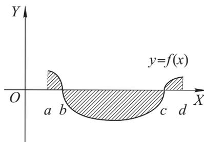
$$S = \int_a^b f(x) dx - \int_b^c f(x) dx + \int_c^d f(x) dx.$$
